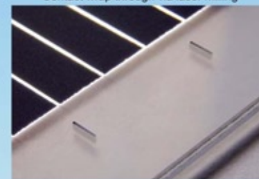
Contact wrap through via laser milling
