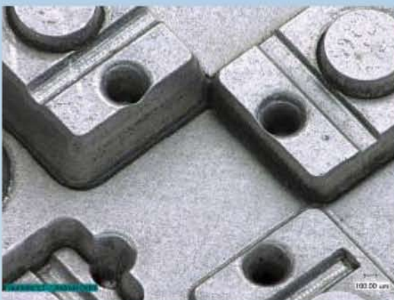
Moulding tools engraved by ps laser
