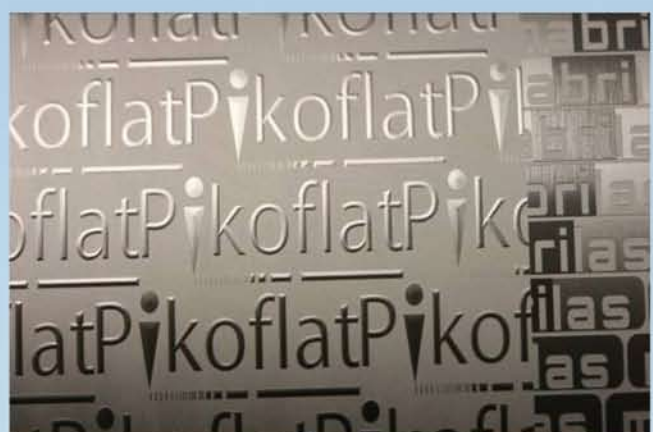
Press cylinder engraved by ps laser
